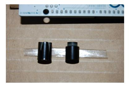
2. The 10mm mounts that Radio Shack sells are metric thread. They sell SAE machine screws. In order to get longer machine screws, you will need to find a hardware store that sells 3mm metric screws.
