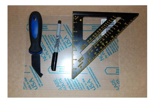
Using a speed square as a guide, pull the cutter across the board to make a groove. Then, snap the material along the groove and take a file to smooth the edges.
